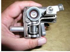
A top view of the unit showing the operating lever in it's assembled location, kept properly located by an e-clip. You can't get the air valve casting off with the operating lever in this position, so...
