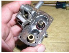
This spring can be left in place unless it falls out. It's often stuck in there good and you don't want to stretch it while removing it. Better to simply clean it by soaking it where it is. That plastic bushing comes out easily.
