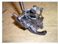
Remove the two pozidrive screws securing the air valve casting to the FASD body...
