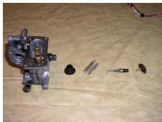
This shows the order of assembly of the air valve, From right (top in operation) are the air valve disk, vacuum piston, outer spring, and plastic bushing.
