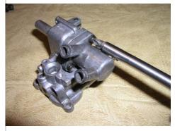
Time to remove the water cell and thermostat bulb. Two more pozidrive screws here.
