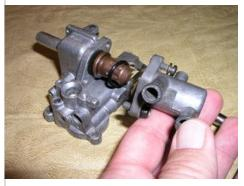
Withdraw the water cell and reveal the thermostat bulb and O ring. Be sure the bleed screw on the water cell is clear. You will need to bleed air from the water cell with the engine running once everything is back together. The thermostatic actuator will not work if there's air in the water cell, and it will not bleed itself. If you find the unit needs to be bled constantly to keep it functioning, you don't have an FASD problem, you have a head gasket problem.
