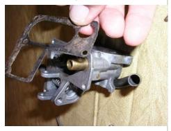
With the operating lever removed, you can remove the gasket safely. Remove the thermostatic actuator return spring, bushing and sleeve.
