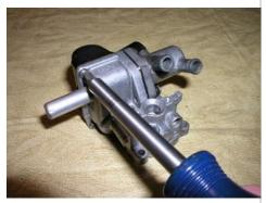
Remove the three pozidrive screws holding the snorkel cover on and remove it.
