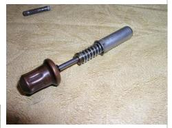
This shows how the thermostatic actuator, bushing, return spring and sleeve interrelate. There is a set screw in the bushing that serves as an adjustment for shutoff temperature. The sleeve has three lugs on it that fit into the FASD body. Experiment with the orientation on reassembly until you get it seated fully. If you were to place this assembly in a C clamp to apply pressure to the actuator rod, then you could test its operation in hot water.
