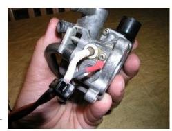
Bottom of the unit showing the cartridge heater. The heater warms the fuel for better atomization during cold starts. It is controlled by a thermostatic switch on the manifold.
