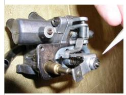
The locking washer and threaded rod should be left alone. This adjustment was set at the factory and should not require attention, and you'll likely break it if you try to. If you feel the need to remove the metering needle from the bracket, gently pry up the black spring clip (no need to remove it) and slide the needle sideways out of the bracket. In most cases, you won't need to do this.
