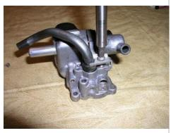
Now remove the pozidrive screw holding the clamp to the outlet tube...
