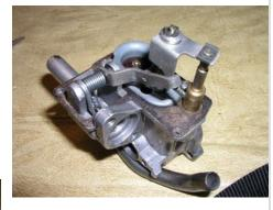
Now slide the operating lever on its pivot to the left (outside) to clear the metering bracket.
