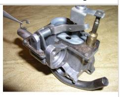
The E-clip removed. The outlet tube is just propping up the unit so it won't fall over while I photograph it.
