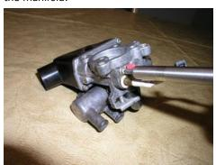
Begin the disassembly by removing the cartridge heater. This gets the wires, which are often brittle, out the way and prevents further damage. Remove the pozidrive screw and the heater should pull out...
