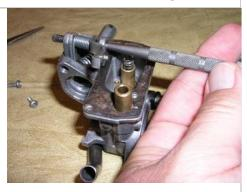
Once the ridged bit at the and of the pivot is clear of the casting, you should be able to remove it by hand.
