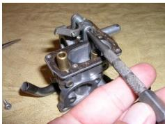
Time to remove the operating lever. Do not attempt to remove the gasket until you remove the operating lever as you will wreck it. With a suitable drift, tap the operating rod pivot from the inside out.
