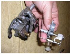
...and remove it from the body. This is as far as you should need to go with disassembling the air valve casting. The
