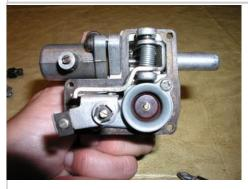
Here are some views of the top of the unit with the cover off. Take note of how the operating lever and needle metering needle/stepped air shutoff valve all interrelate.
