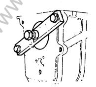
17. Remove reverse gear shaft.
