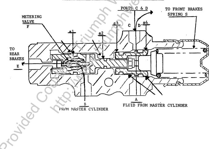
FAILURE SENSITIVE PRESSURE REDUCING VALVE
